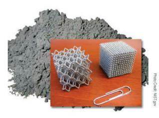
(above) Metal powder and resulting product using laser powder bed equipment. (below) DMLS, one of several metal additive techniques, leads to light-weight, low-production volume parts .
