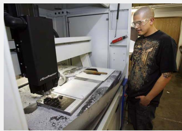
CNC operator Jefferson Duran, who has worked at Accurate Dial and Nameplate, Inc. for three years, cuts a nameplate with a micro-milling machine in Glendale on Monday, April 25, 2011. (Tim Berger/Staff Photographer)
