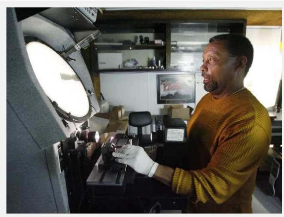
Roy Adams, in quality control, creates a mold of a part so he can measure how precise a part was machined at Centerpoint Manufacturing Company, Inc, in Burbank on April 26, 2011. (Tim Berger/Staff Photographer)
