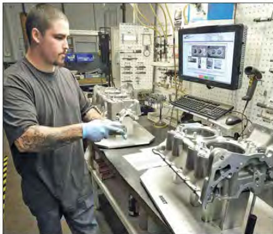
■ Top: Nicholas Jolly gives a final inspection to the crank case of a piston engine at B&B Manufacturing in Valencia. Right: Final inspection of flight control parts. Photos by Dan Watson.
