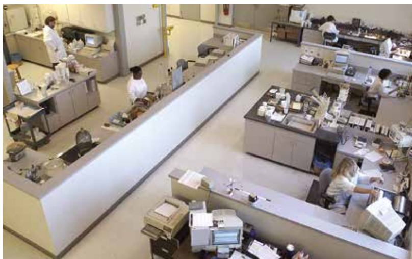
To ensure our customers receive the most reliable and consistent products available, Whip Mix tests every batch of gypsum for setting time accuracy, consistency, setting expansion and strength.
