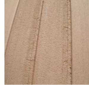
Poorly extruded "composite decking"
