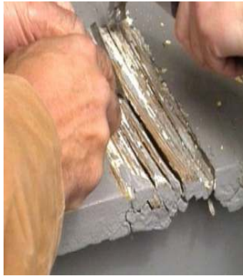
Douglas fir splitting and cracking
