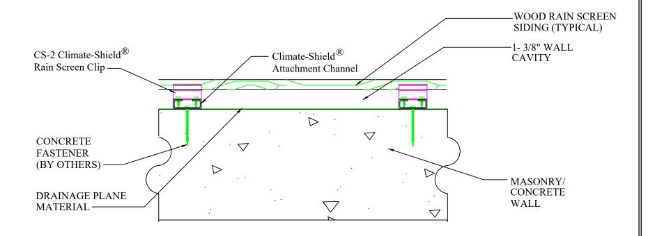
Typ. Concrete Wall System, Plan View
