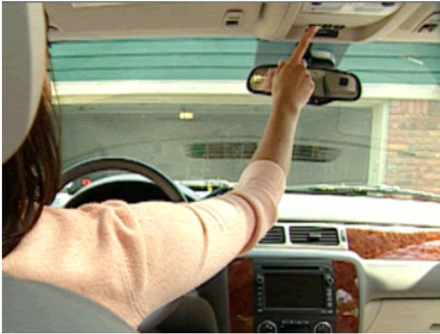
To program another rolling code device such as an additional garage door opener, a security device, or home lighting, repeat steps 1-4 substituting a different function button in Step 3 than what you used for the garage door opener. For example, you could assign the left-most button to the garage door, the center button to a security device, and the right-most button to another garage door opener.
