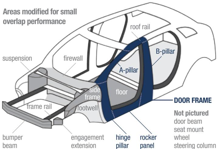
this happens the dummy experiences less change in velocity but ends up further to the left side of the vehicle, increasing the risk that the head could miss the front airbag if the safety belts and airbags aren't modified to better control the dummy's movement.
