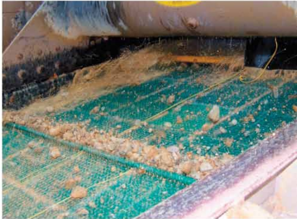
The success of Polydeck’s Maxi screen panel design at Fairmount Mineral’s Menomonie plant convinced management to use the same approach at Maiden Rock.
