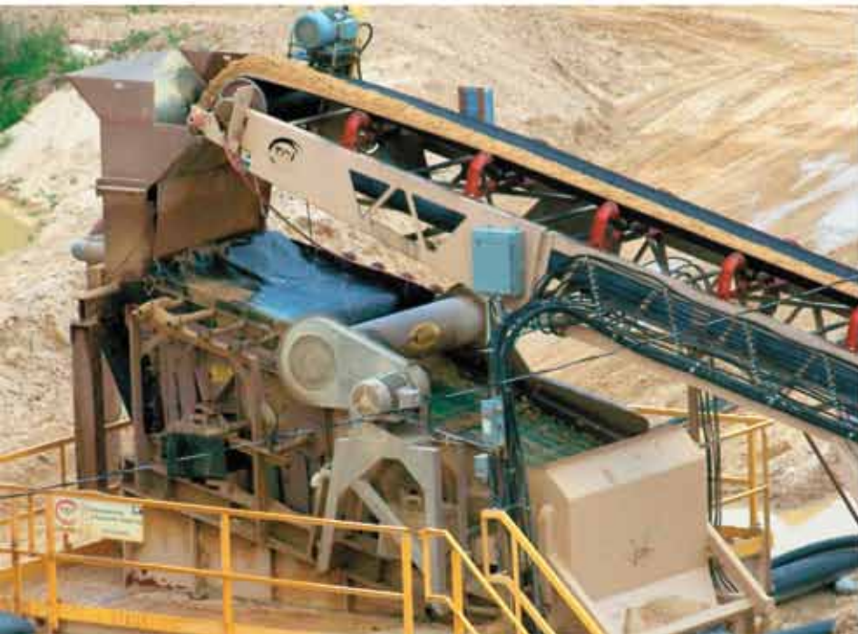
For increased efficiency and throughput, the Menomonie operation uses Polydeck Maxi panels on its double-deck scalping screen.
