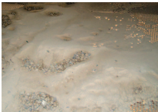
Figure 1: Wire cloth screen is blinded over at Hanson's Santee plant.
