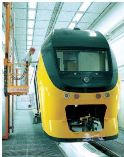
This well-established manufacturer of rail cars received state-of-the-art paint work systems for the use of water-based paint. The combination spray and drying booths with recirculation air systems are low maintenance and have an effluent free paint particulate scrubbing system.
