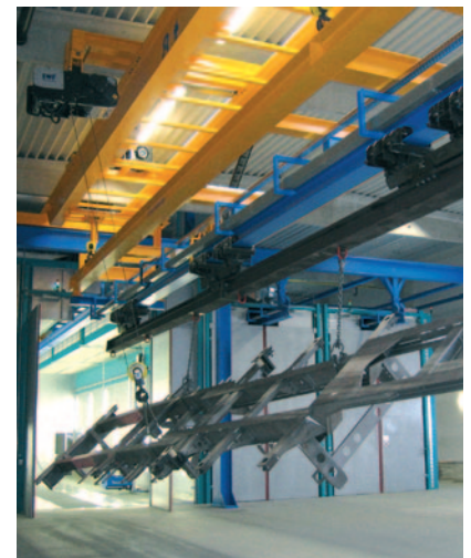
Large booth with dry separation and integrated exhaust air heat recovery system for coating of container chassis, flat bed trailers and semi-trailers according to specific customer requirements.
