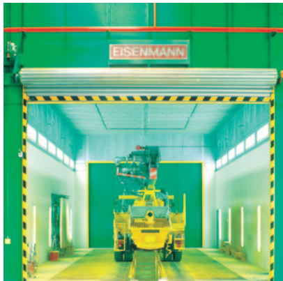
Combination large capacity spray booth for the global market leader in mobile concrete pumps.
