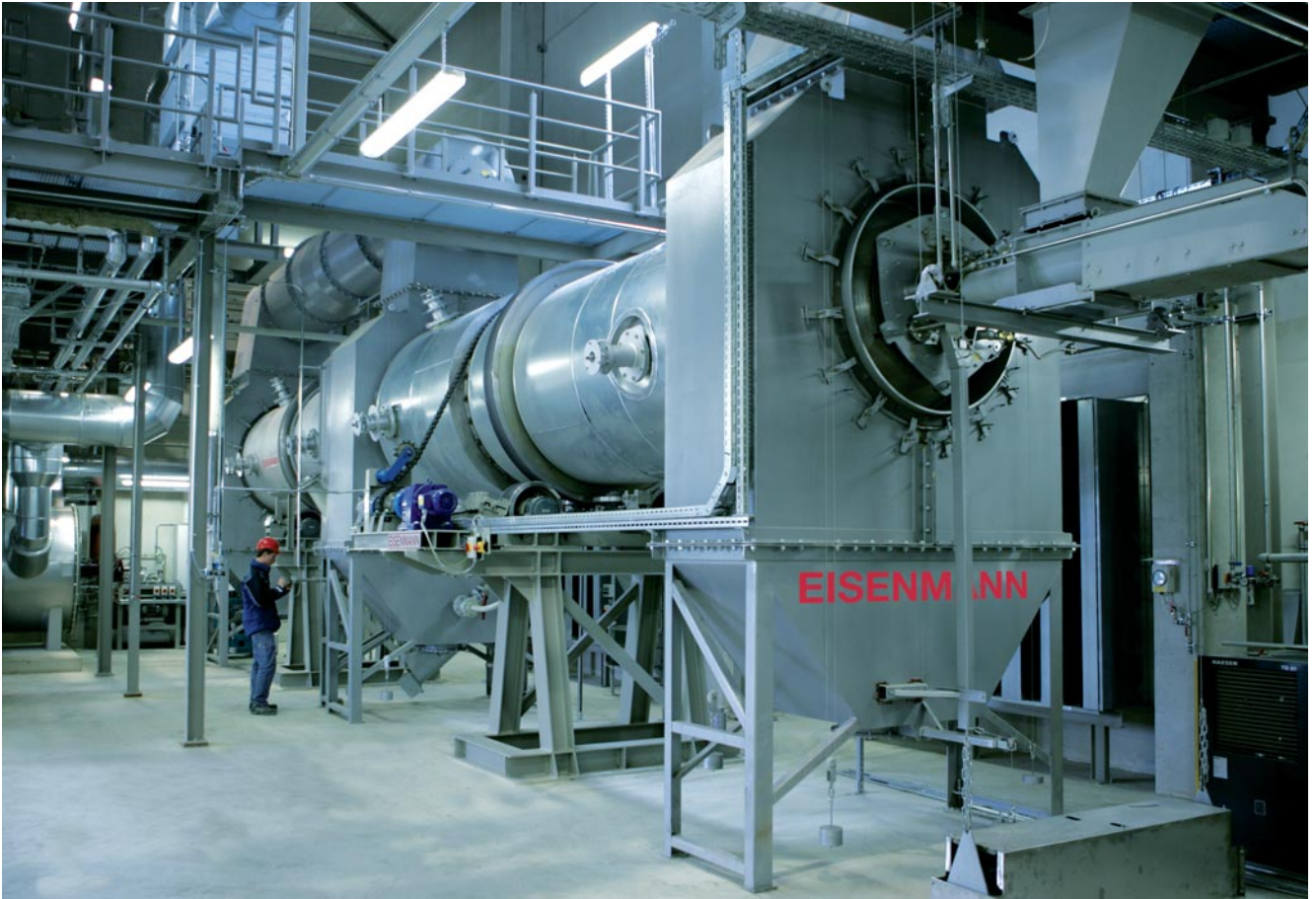
Picture 5: The continuously working Pyrobuster® designed for a throughput of 650 kg dried sewage sludge granulate with approx. 88% DM per hour.
