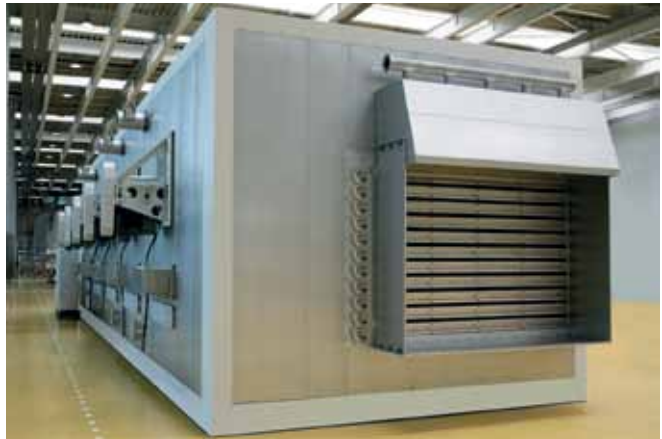
Oxidation oven vertical down.
