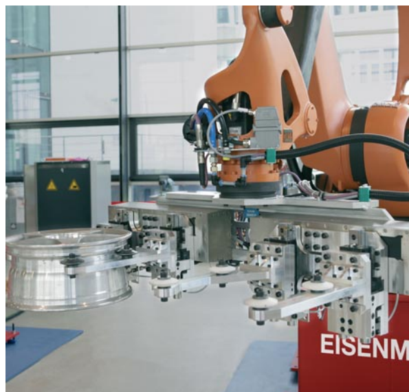
Automatic transfer with individual designed grippers mounted on robots
