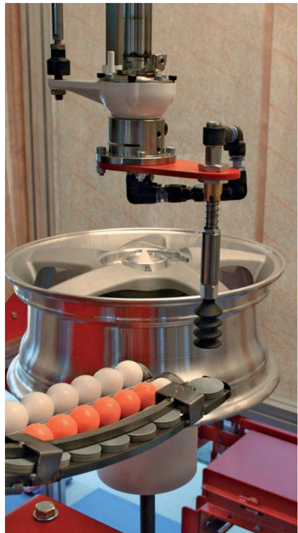
Automated masking of bolt holes with balls or taps
