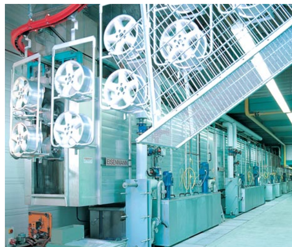
Pretreatment plant for chromium-free conversion treatment
