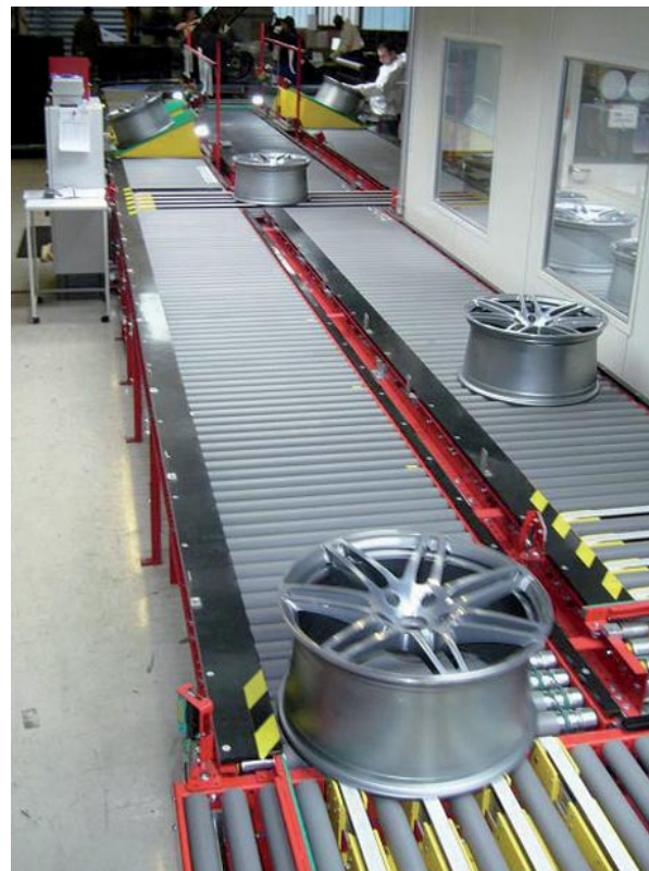
Final inspection with two separate tilting tables for optical inspection of the wheels
