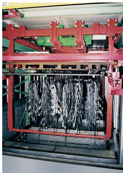
Easy Coater System E-coating parts for a heavy truck manufacturer
