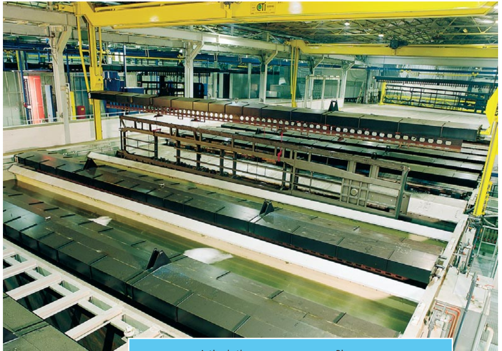
Photo above: The cleaning and pretreatment baths are completely integrated into the painting process with a programmable hoist system.
