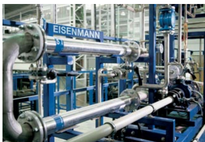
Highly effective cleaner bath recycling through ultrafiltration.
