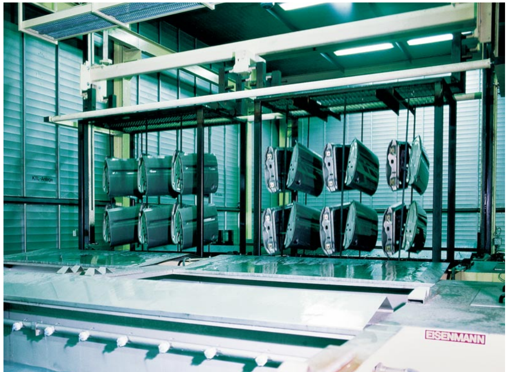
Photo right: Cathodic E-coat system for automotive parts using a 10-stage pretreatment.
