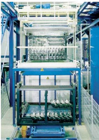
Cathodic E-coat system with flexible programming at a custom coating house.
