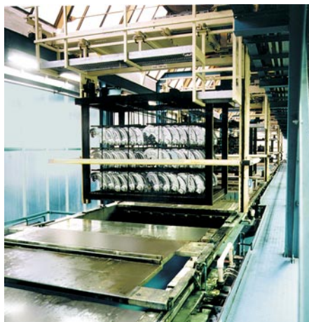
Cathodic E-coat with programmable hoist for automotive parts.
