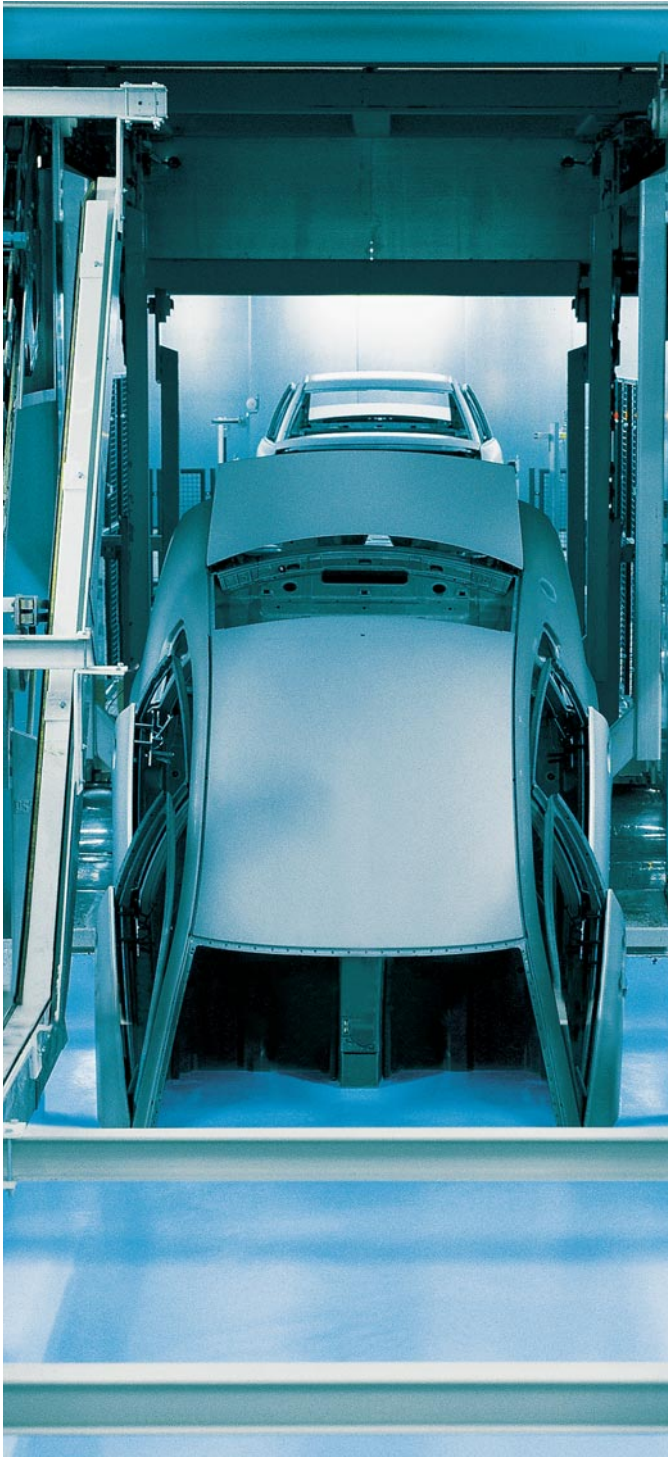
Photo left: Continuous E-coat system using a pendulum conveyor in the automotive industry.
