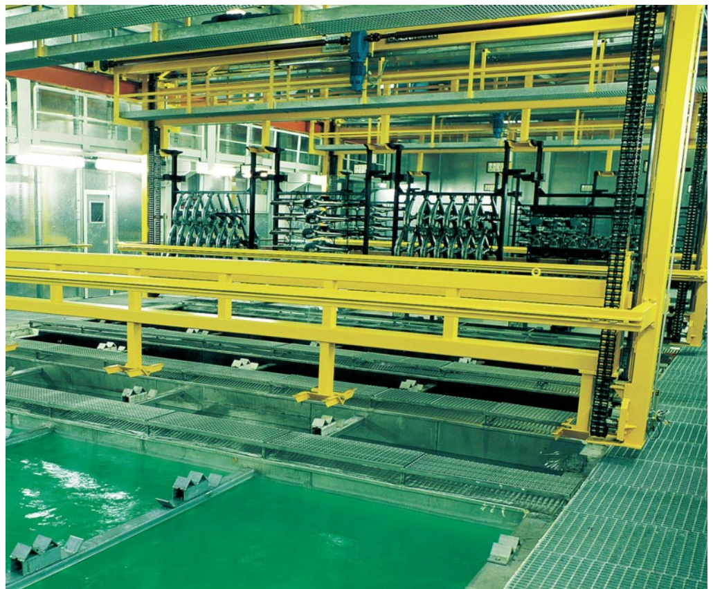
Programmable hoist dip lines allow individual processes for small batches and large work pieces.
