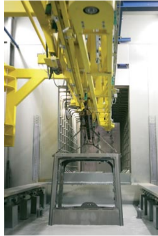
Photo left: Cathodic E-coat system with overhead chain conveyor and special lift station for truck cabs.
