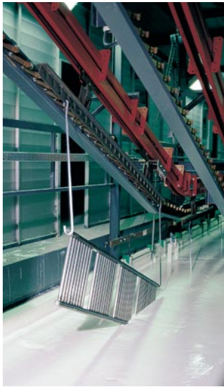
Continuous dip painting is the most frequently used painting process for radiators.
