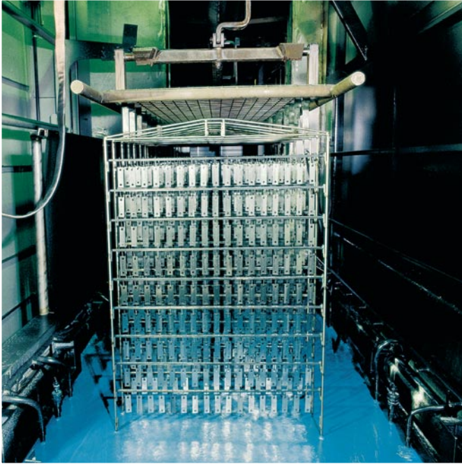
Photo above: This custom coating business uses the advantages of an indexing cathodic E-coat system for individual batches.
