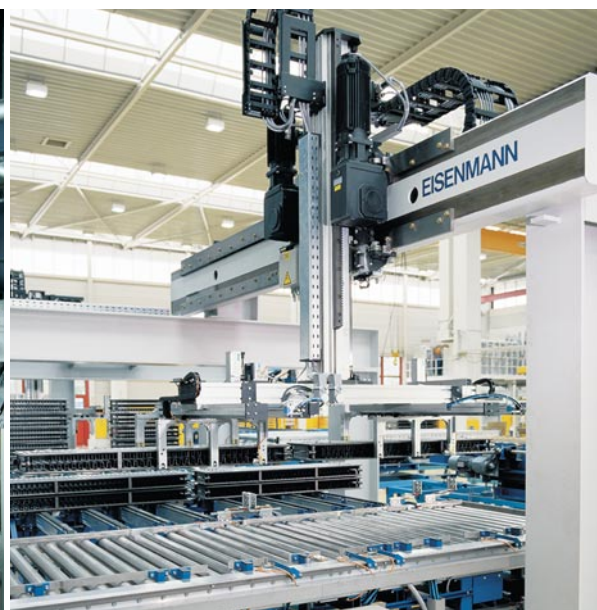
Radiator painting: Dual-rail gantry robots unstack the parts and load the paint line
