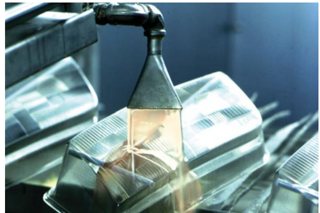
Flow coating facility for the scratch-resistant coating of diffusing screens made of plastic
