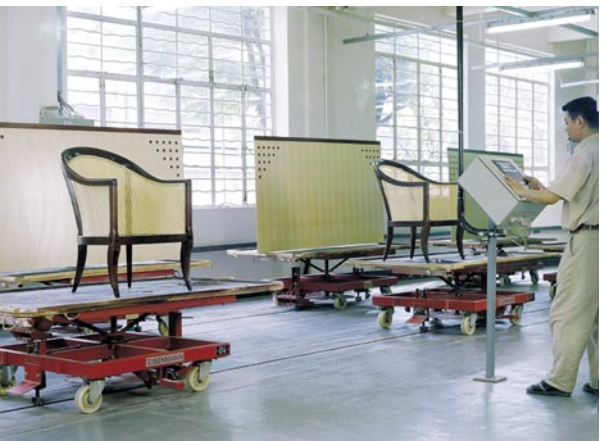
Furniture paint line with underfloor conveyor system
