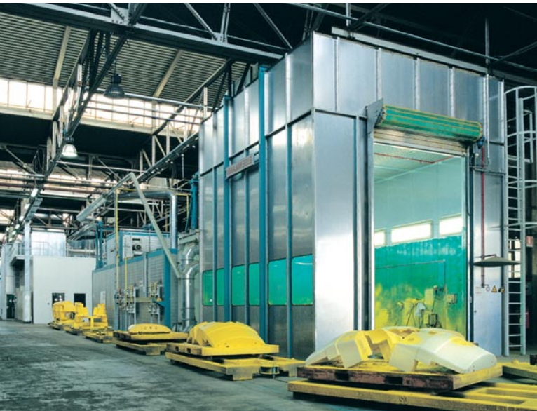
Wet-spray system for forklifts
