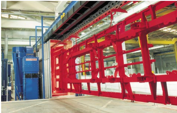
Combined E-coat and powder coating system for truck frames
