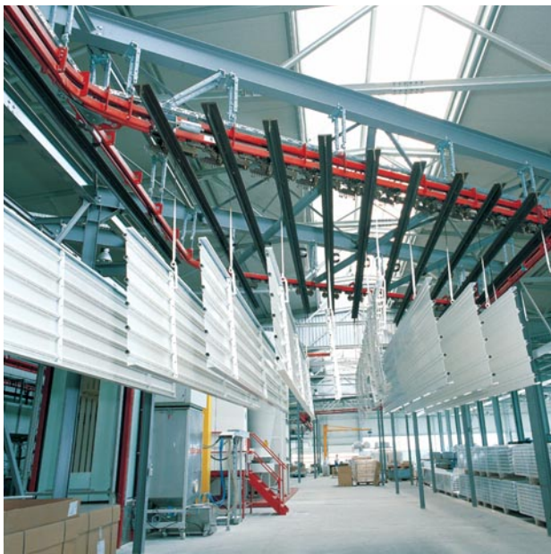
Top: Power & Free conveyor for destination controlled transport and stacking in the cross buffer in the smallest available space
