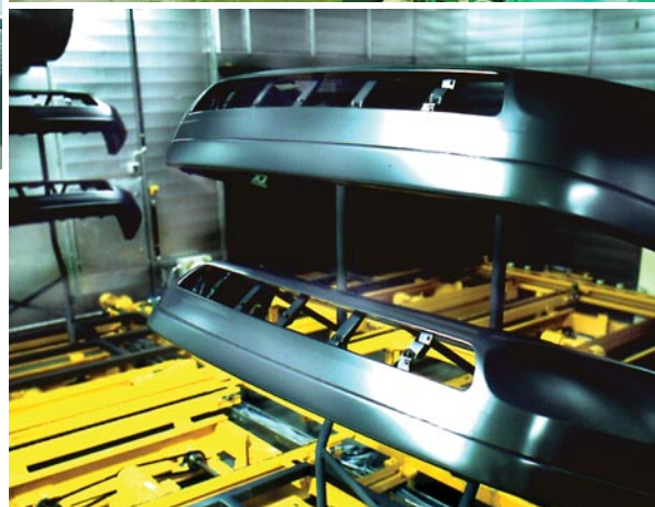
Top: Power & Free conveyor for destination controlled transport and stacking in the cross buffer in the smallest available space
