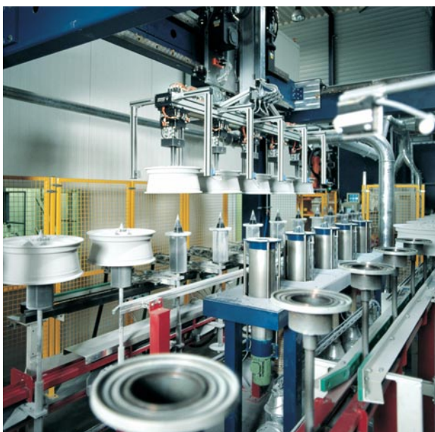
Gantry robots loading the painted parts onto the spindle conveyor of the powder curing oven
