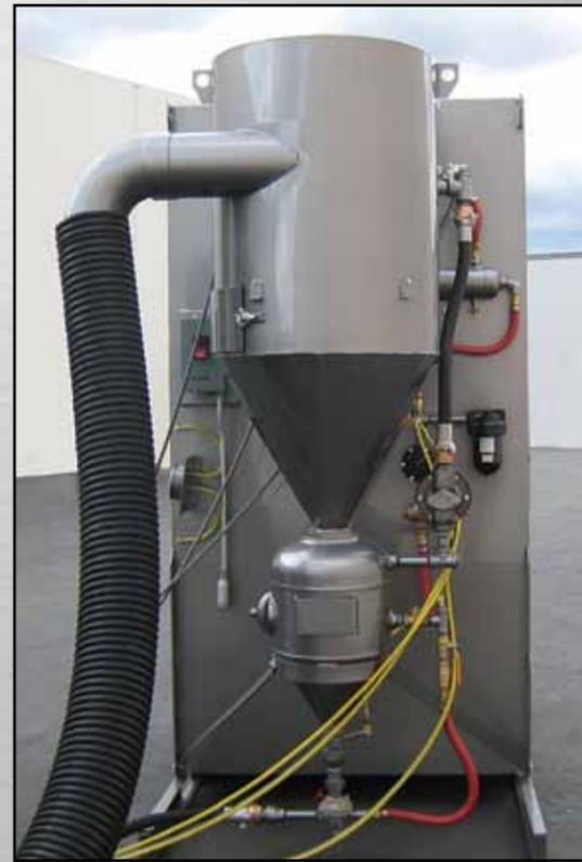
The 7-inch diameter hose and massive cyclone prove this baby sucks! Generous pressure vessel gives tons of blast time even with large nozzles.
