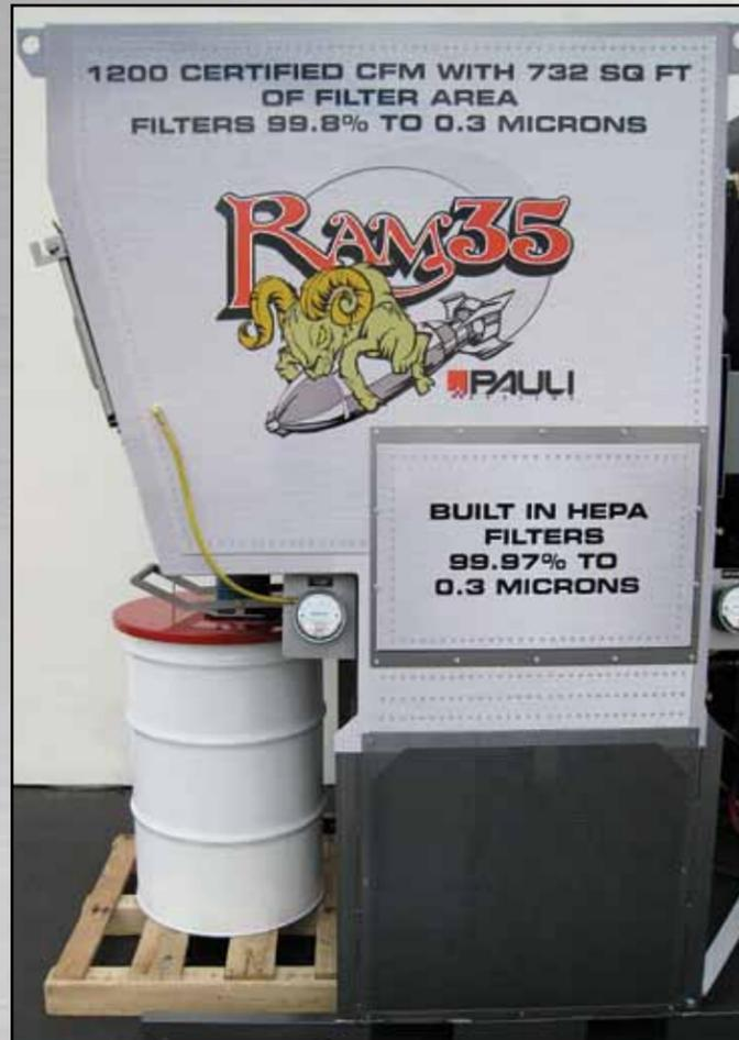
RAM 35 dust collector features 20 air changes per minute in the blast enclosure, 1200 Certified CFM and optional HEPA filtration.
