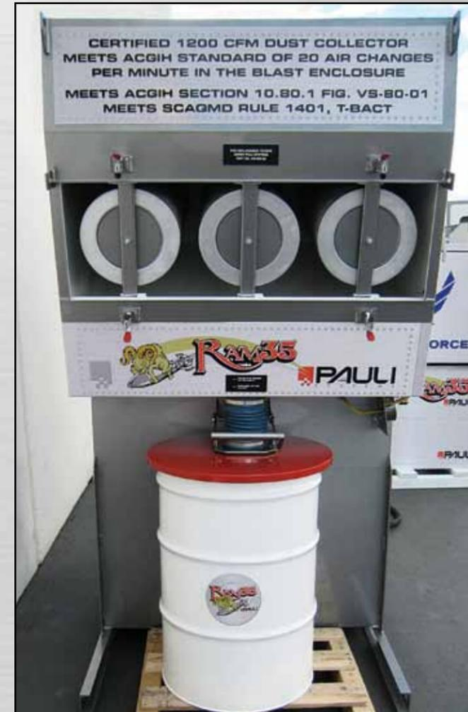
Three banger dust collector with locking dust discharge lift handle and lid; easy change dust drum; no messy dust drawer. Handle and lid included; 55 gallon drum not included.
