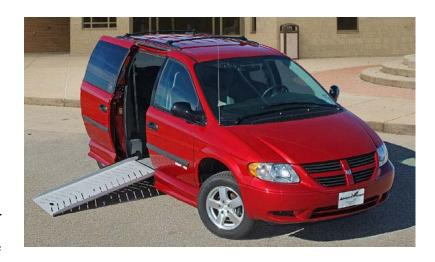
Inside, Q-Straint tie-downs provide greater security and are located for maximum value. Wide passenger side and driver side sliding doors offer convenient, easy access for all. Amerivan conversions feature lowered rear seats and front seats which can be easily removed.
