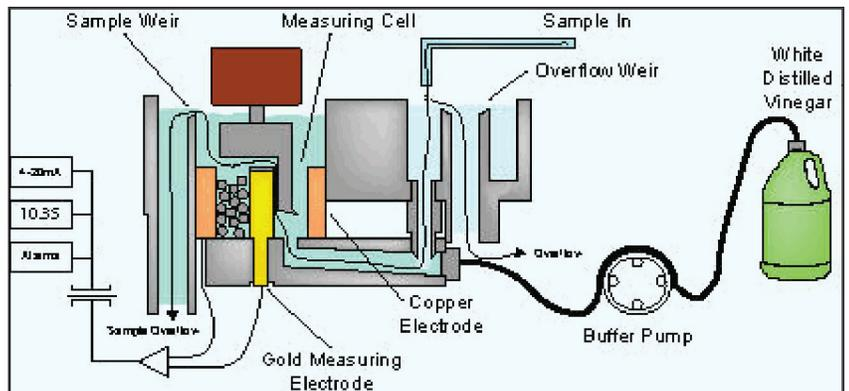
The sample stream runs down through the lower block, where it mixes with vinegar (and potassium iodide where total chlorine is being analyzed), and then flows upward through the measuring cell. Within the cell, the vinegar provides pH buffering to a value of 4.0, and aids in keeping the cell clean.
