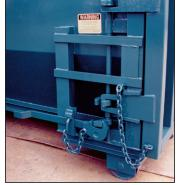
for easy operation. Handle is secured by a ¾" solid pin, 180° turn keyway locking system.
