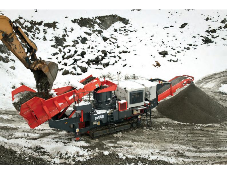
The QH440 is a tracked, self contained cone crusher with an on board diesel engine.
