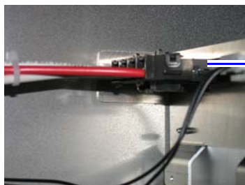
Figure 28. Grommets installed in sign section pathway openings.
