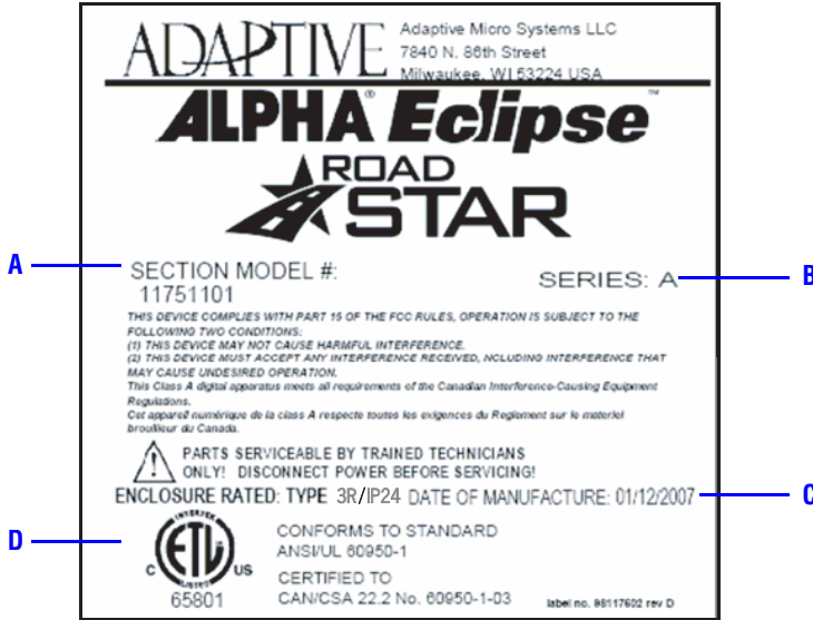
Figure 15. Section compliance labels are located on the back of each sign section
