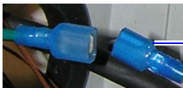
Figure 29. Cable connection between sign sections.
