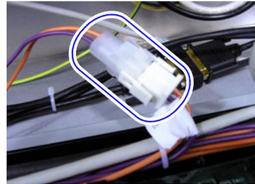
Figure 9: Disconnect the power cables
