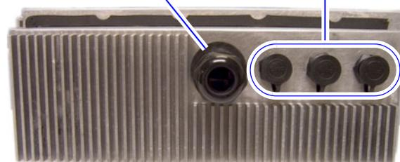
Rear view of controller (identical for both series) on the back of the sign's controller section (bottom right-most case).
