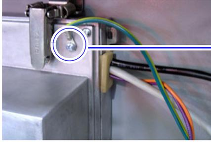
If present, remove the ground wire screw with a Phillips-head screwdriver to disconnect the grounding wires.
