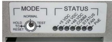
Figure 12: Toggle or rocker switch.
