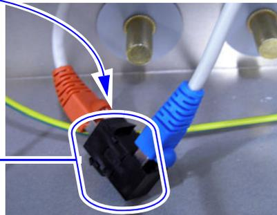
If present, leave this coupler attached to the cable inside the sign.
