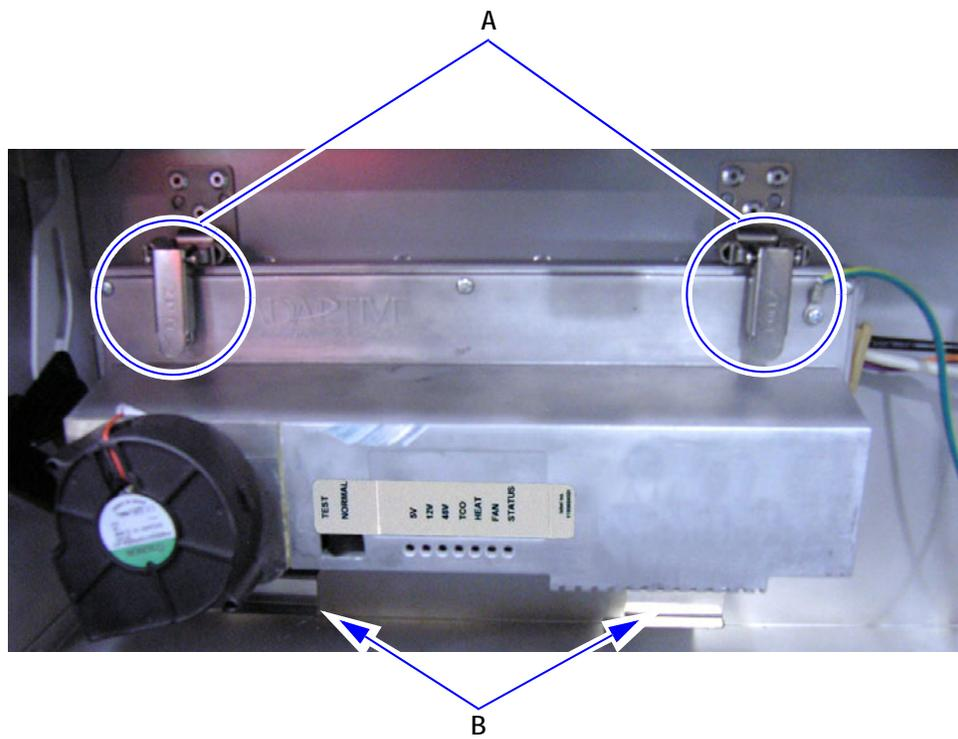
Figure 10: Release the latches holding the controller in place
