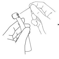
Use the nozzle needle **Mat. no. 0.410.0921** to free the water passage in the spray nozzles.
