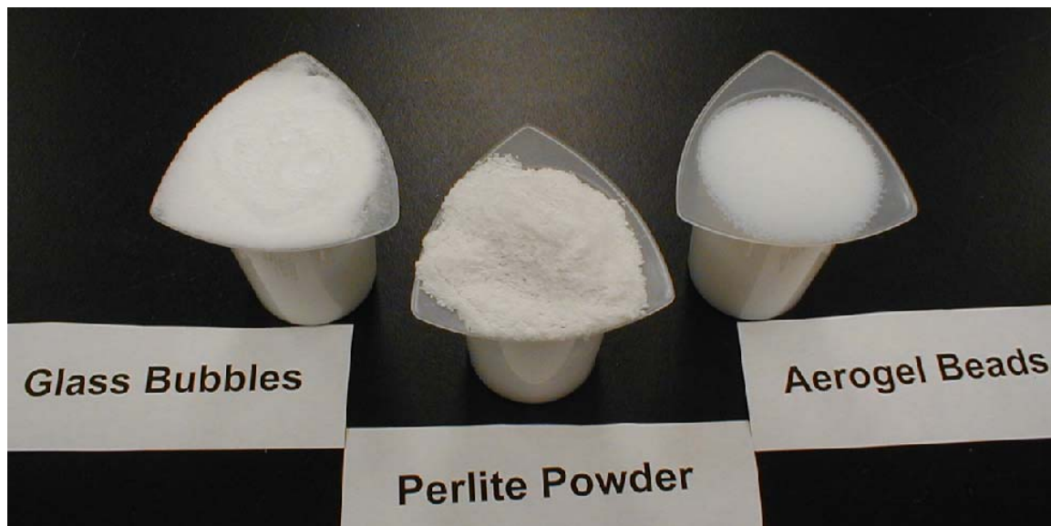
FIGURE 3. Different cryogenic insulation materials in the bulk-fill form.
