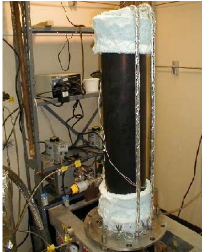
FIGURE 1. Cryogenic insulation test apparatus for cylindrical specimens with vacuum can removed.
