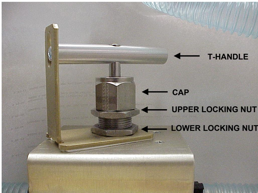
5. Turn the handle counterclockwise to decrease the adjustment. This prevents overpressure for the next step. This is usually only required for first time adjustment.
