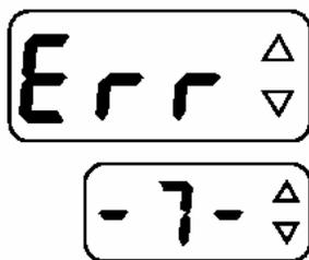
Sensor faulty. Remove sensor from use and replace.
