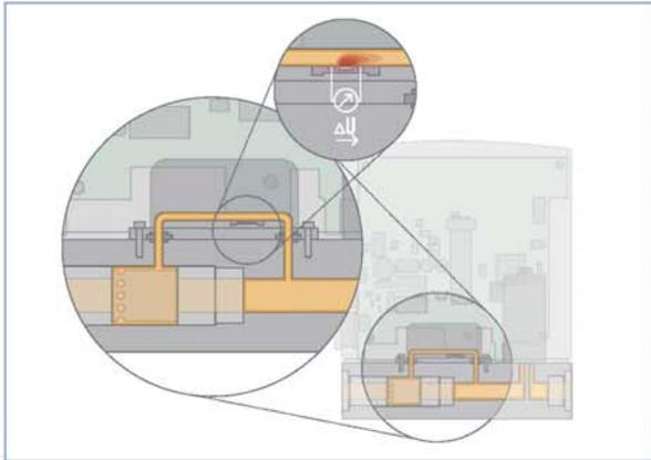
The actual flow rate is detected by a sensor. This operates according to a thermal principle which has the advantage of providing the mass flow which is independent on pressure and temperature.
