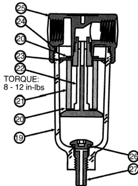
**Caution: Shut off air supply and exhaust the primary and secondary pressure before dis-assembling the unit. (Units may be serviced without removing them from the air and nitrogen lines.)**
