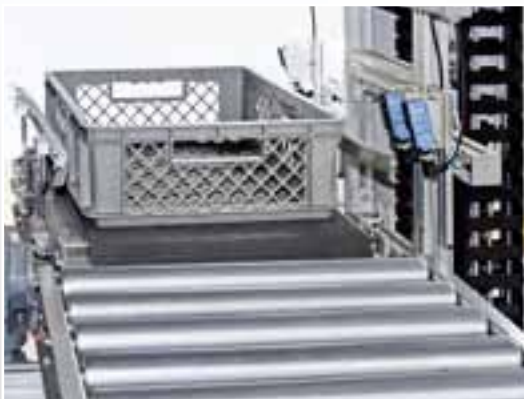
Transfer from belt conveyor on lifting carriage to the subsequent roller conveyor
