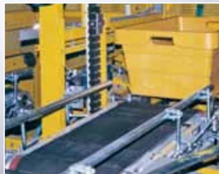
For unit loads of identical dimensions, the platforms are suspended from the rubber block chain and run in plastic guide rails for the entire circuit. This ensures smooth vibration-free running.
