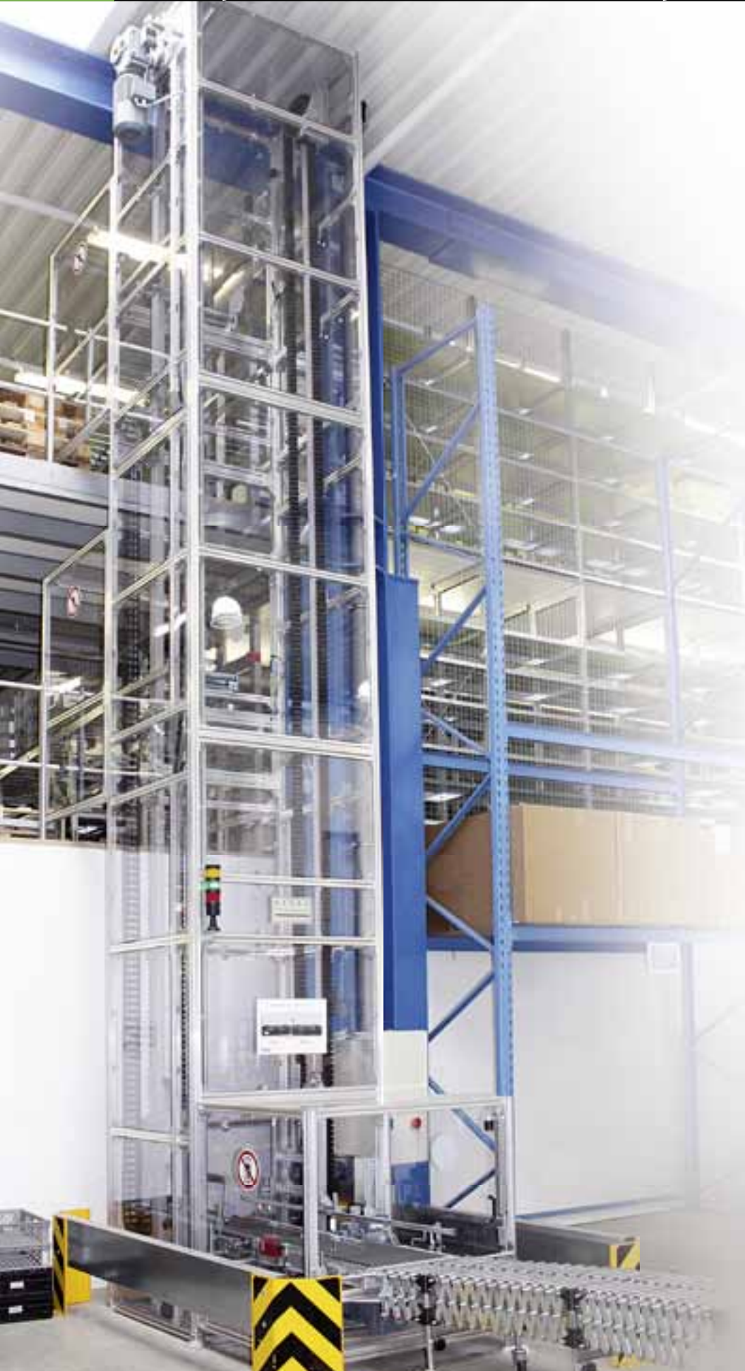
Feed station of a portal lifter with transfer onto the pivoting infeed conveyor, separating out the items.
