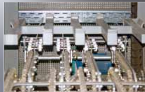
For unit loads of varying dimensions the platforms are designed in the form of a rake.
