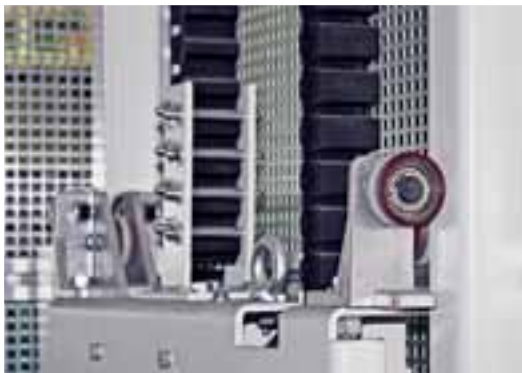
Vulkollan rollers guide the carriage
