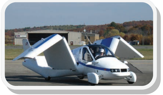
Terrafugia's Transition as it prepares for flight mode with the unfolding of its wings.
