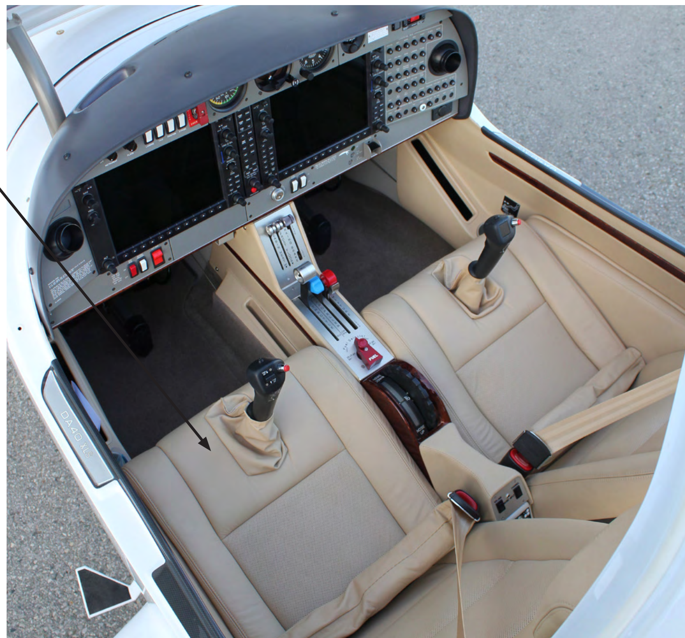
The remolded trim wheel cover and narrowed seat buckle area increases the width of each seat by 1 inch. A mini-pocket on the pilot inboard side panel conveniently stores smart phones or electronic devices.
