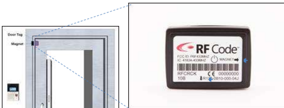
Figure 3 - Door Tag and Magnet Position on Closet Door
