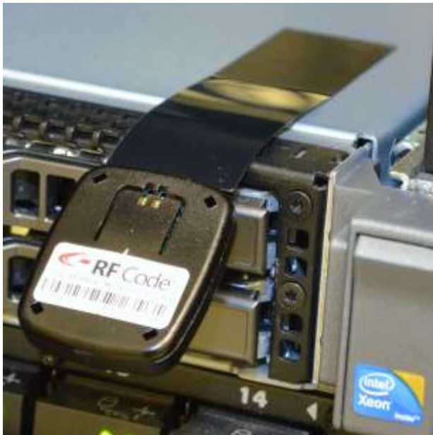
M174-i with Flag tab, installed on server
