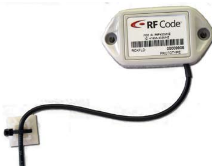
Figure 5: Strain Relief Wire Mounting Method
