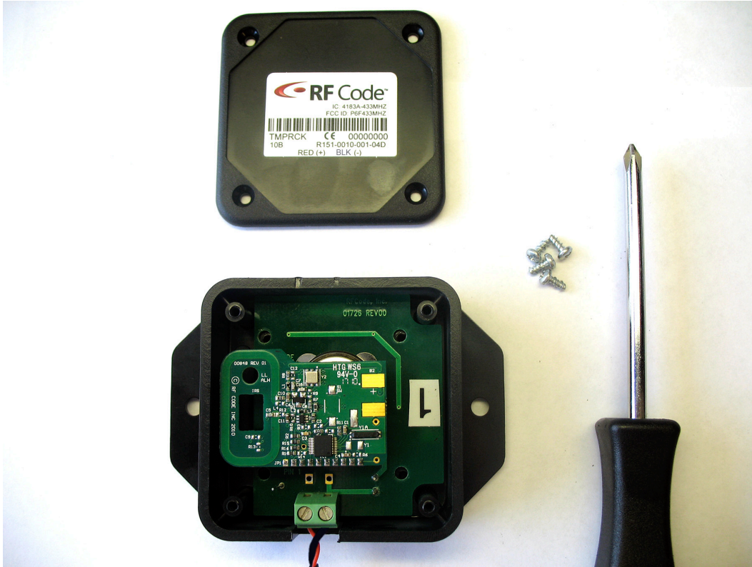
Figure 8: Remove screws holding tag board in place
