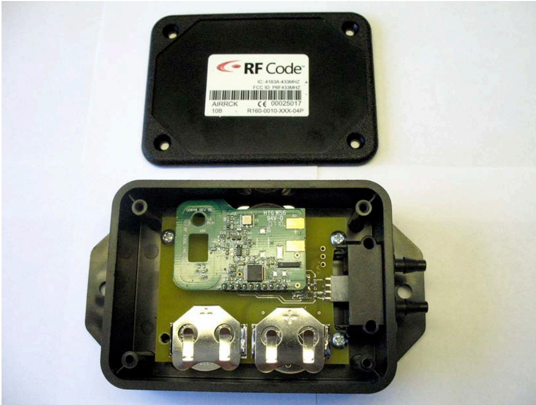
Figure 5: Remove tag case cover
