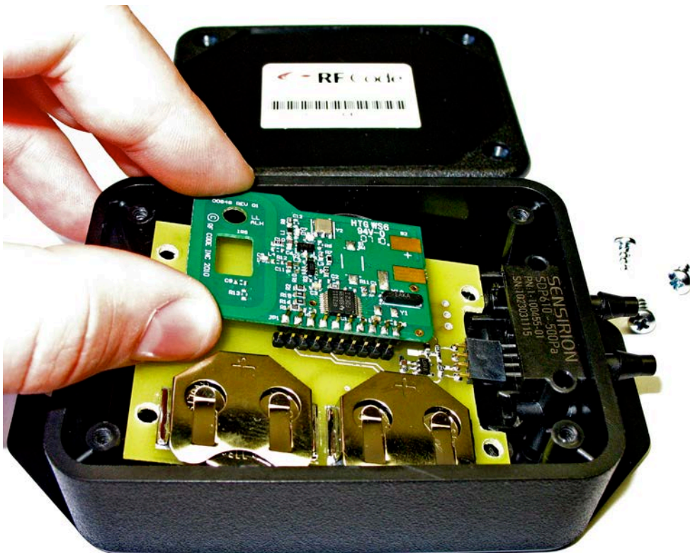
Figure 8: Remove tag board from the case
