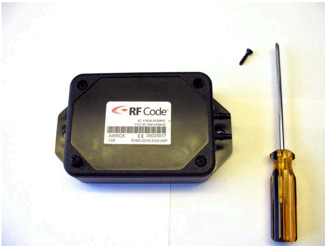
Figure 4: Remove screws from R160 Tag Case
