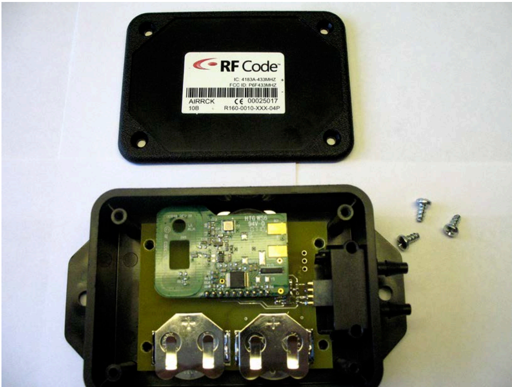
Figure 6: Remove screws holding tag board in place
