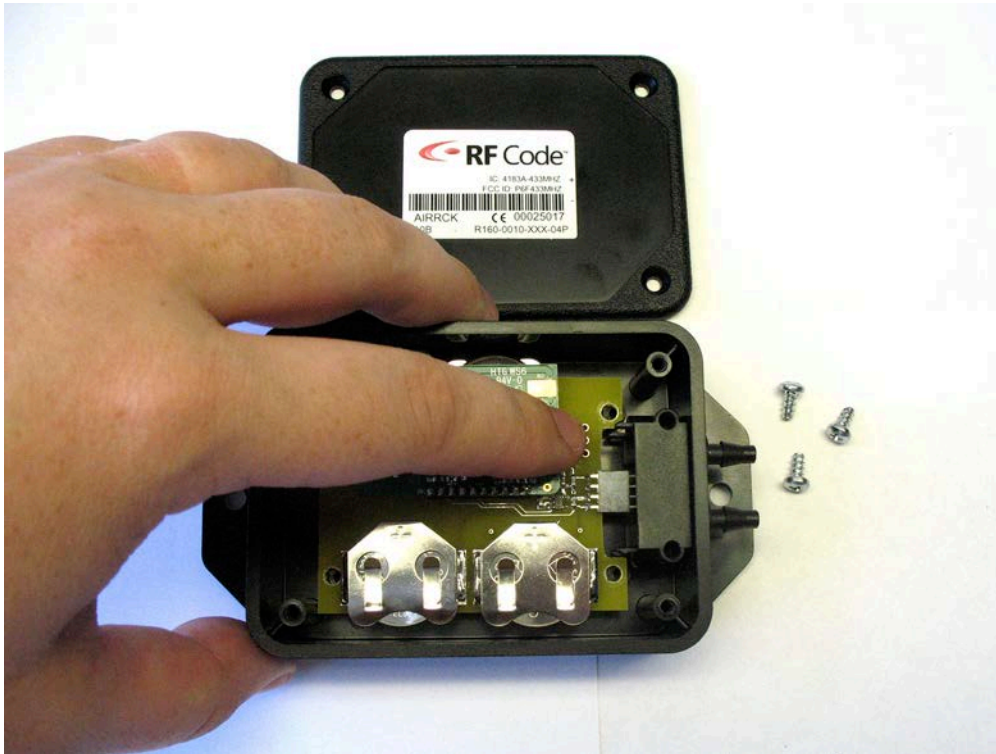
Figure 7: Slide the tag circuit board to the left
