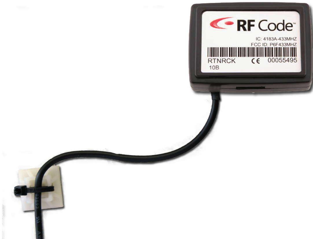
Figure 4: Strain Relief Wire Mounting Method
