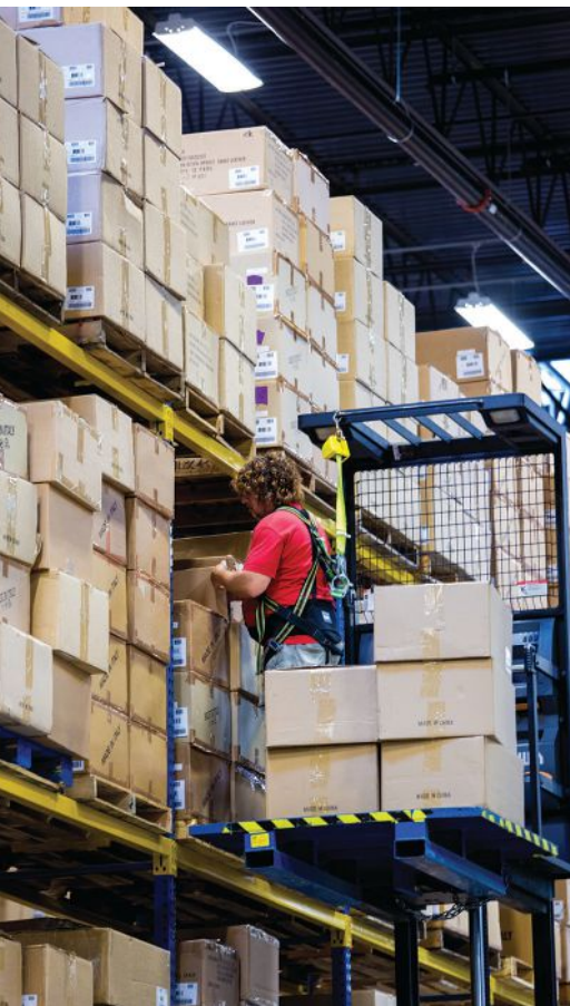
Order picking lift trucks are used for carton putaway and picking (top left). Below, an associate picks replenishment orders from a mobile robot (bottom right).
