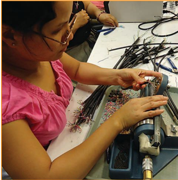
All assemblers are cross-trained to perform wire stripping, potting, heat-shrinking, soldering, connector termination, horizontal overmolding and testing. Photo by Jim Camillo
