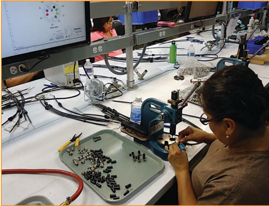
A computer monitor within each station displays drawings of the cable component or components to be assembled, along with specific assembly instructions. Photo by Jim Camillo
