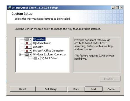
Select each feature to install/uninstall by clicking on the icon next to that particular module and choose "Will be installed on local hard drive". Click "Next" to proceed.
