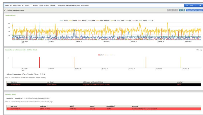
Take data from multiple sources (top chart) and cross-correlate it to see what systems were impacted together to cause such a big anomaly score
