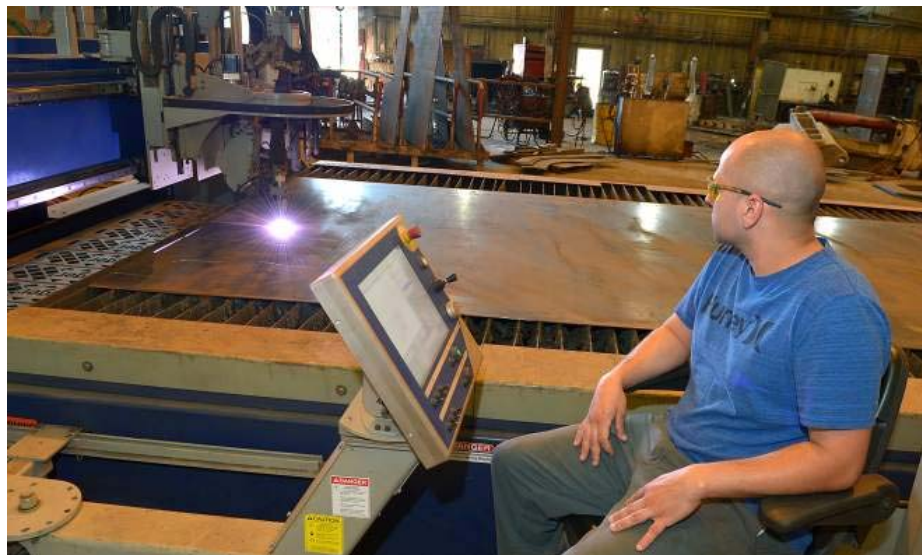
Advocate staff photo by PATRICK DENNIS -- Robert Rogillio monitors the work done at a computerized burning table, which cuts sheets of steel into designated shapes at the Anvil Attachments plant in Slaughter.
