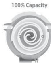
efficiency and humidity control. Based on demand, the modulation ring is activated, sealing the bypass ports and instantly shifting capacity to 100%. Take advantage of "shift on the fly" stage changing (no stopping and starting required like other two-stage compressors).
