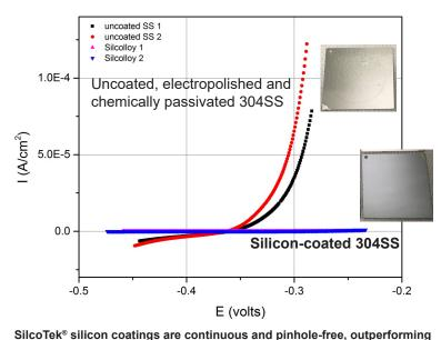
electropolished and passivated stainless steel in corrosion testing.
