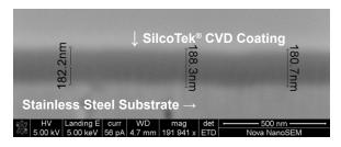
SilcoTek® CVD coatings are thin, flexible barriers that increase the lifetime of critical components in corrosive environments. The coatings are typically less than 2µm thick.
