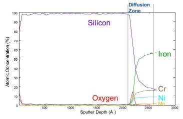
SilcoTek® coatings are comprised of hydrogenated amorphous silicon (a-Si:H), enhancing the chemical inertness of stainless steel.
