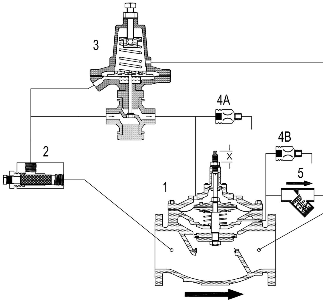
1. Main Valve - Model 106 or 206-PT-EF c/w X102 Stroke Limiter.
