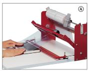
Slightly tighten the film and cut it off with the built-in knife.
