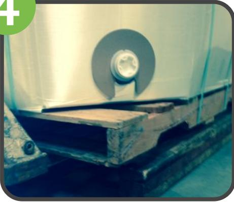
Place the pallet on an elevated sturdy block or boards. Make sure you choose something that can support the weight of the tote, because it will remain in this location until the tote is empty. The height can be any level you choose, but the goal is to allow the oil inside to gravity feed out of the hose. This example tote is elevated 4-5" off the ground.
