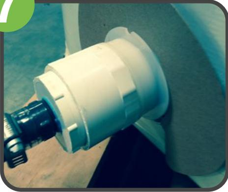
With the cutter facing in, screw the white fitting in on top of it. The hose will turn with the fitting as you screw it in, as it is all one piece. Screw this fitting in all the way, until it bottoms out.
