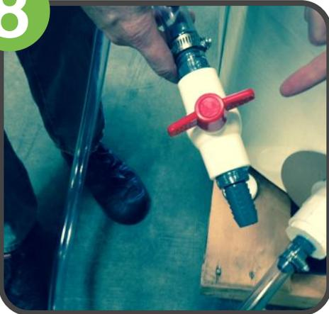
As you screw the fitting in, the cutter will pierce the tote bag and oil will begin running into the clear tubing. Once the attachment is all screwed in, simply turn the valve and oil will begin to flow into your desired container.
