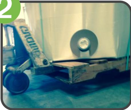
To use this tote dispensing attachment, you'll want to elevate the tote to allow the oil to gravity feed out. One common way to do this is to store your pallet on a pallet rack or shelf. Another is to elevate it a few inches off of the ground. To complete this, first lift the pallet up using a pallet jack or fork lift.
