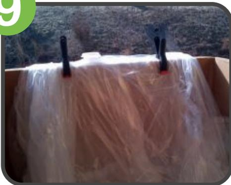
As the bag empties inside of the tote, pull up the bag and clamp it to the edge to allow oil to drain down towards the lower drain fitting.
