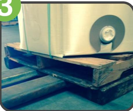
Once elevated, slide sturdy boards under two outer edges of the pallet. Remove the forks of the pallet jack, and reinsert underneath the pallet itself. The boards will keep the pallet elevated to allow the forks to reach underneath.
