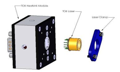
\*Laser plugs into heatsink module
