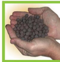
Taconite pellets like these are produced at the Minntac plant and shipped to steel mills to be melted down into steel.
