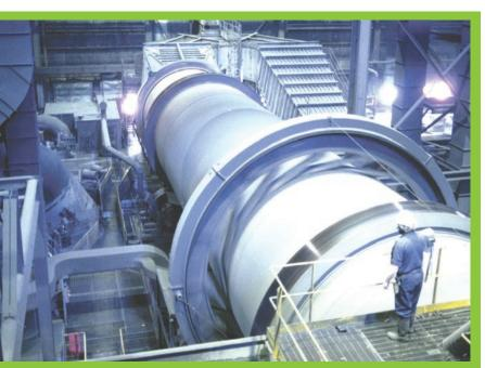
Process lines in the Minntac plant serve kilns that heat a mixture of taconite powder and clay at 2,450°F to create taconite pellets. After installing a high-efficiency burner in one of their process lines, Minntac saved \$760,000 and 95,000 MMBtu in natural gas.
