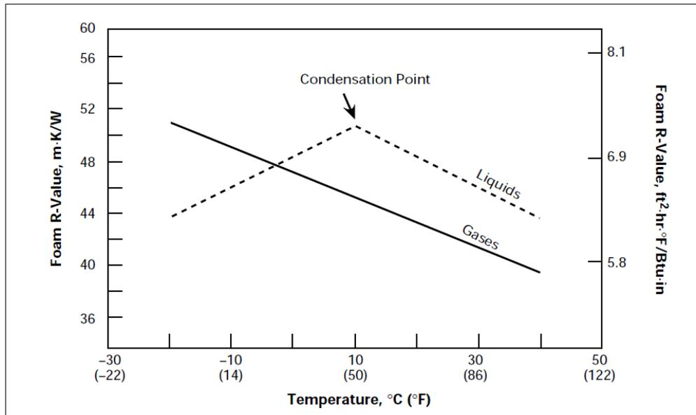
**Figure 2. Foam Insulation Value vs. Temperature for Liquid and Gaseous Blowing Agents<sup>1</sup>**
