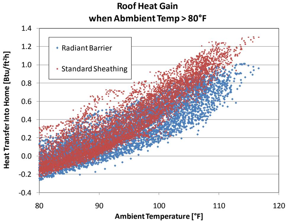
Figure 6. Heat gain into home through each bay monitored (Btu/ft<sup>2</sup> h).
