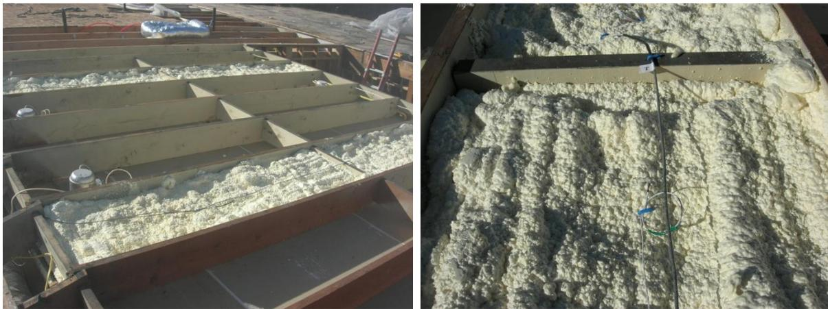
**Figure 3. Thermocouples installed in each test bay on top of the closed cell foam, beneath the roof deck.**
