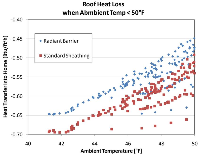
**Figure 7. Heat loss from each bay monitored (Btu/ft<sup>2</sup> h).**
