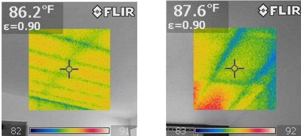
Figure 1. Interior infrared images of the roof before retrofit work. Exterior temperature was approximately 110°F.
