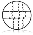
Pads – A rubber part used as an anti-vibration device.
