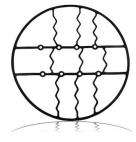
Inclusions – Particles of foreign material (such as oxides, sulfides or silicates) in steel as cast.
