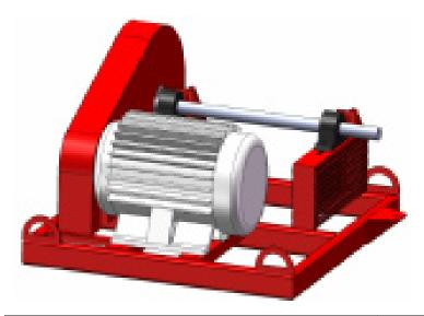
Description. SRS Crisafulli Electric-PTO Power units have industrial duty TEFC (totally enclosed, fan cooled) electric motors mounted on heavy duty skids, equipped with belt and sheave speed reduction (540 RPM resultant speed unless otherwise specified), sheave guard, hitch jack, dual rear stabilizers, ball hitch, intermediate power shaft, and auxiliary pump hitch plate. Performance Range: Horsepower 25 - 250.
