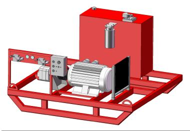
**Description.** SRS Crisafulli electric - hydraulic power units have totally enclosed, fan cooled electric motor mounted on industrial duty skids, with a heavy-duty hydraulic pump, suction screen, fluid reservior, fluid level gauge, fluid system pressure gauge, temperature gauge, breather/ fill cap, ten micron return line filter, flow control valve, pressure relief valve (set at 2000 PSI), fluid cooler, cooling fans. Performance Range: hydraulic output 15 - 150 GΡM.
